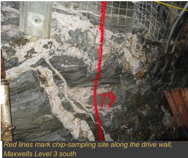
*Red lines mark chip-sampling site along the drive wall, Maxwells Level 3 south*
